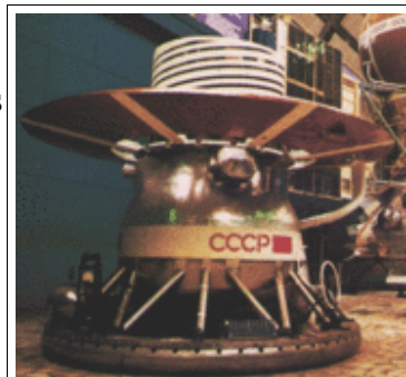
The Venera 13 Lander, which made scientific measurements and pictures from the surface of Venus.
